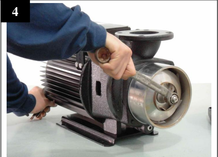
Using wrench to loose the lock nut.
