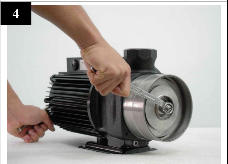
Using wrench to loose the lock nut.
