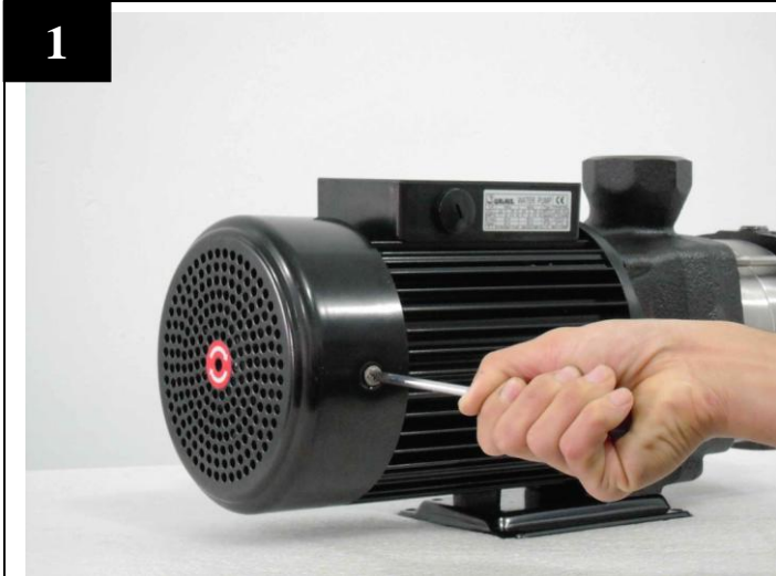
Loose the screws and remove the motor fan cover.
