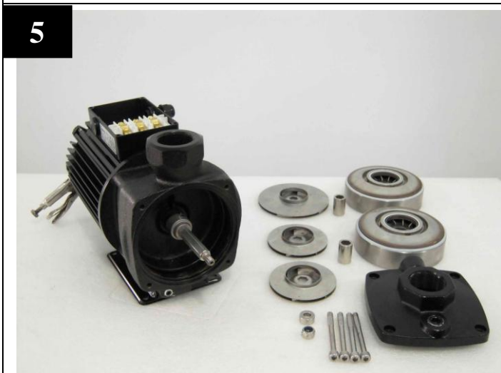
Remove all impellers, sleeves and inter-mediate chambers and place them in order.
