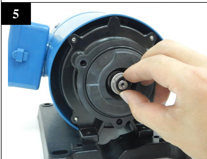
5 Put on the rotary part of mechanical seal
