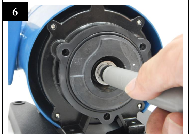
6 Press in the rotary part.
