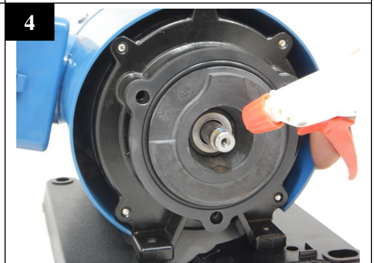
4 Spray water on the shaft as lubrication.
