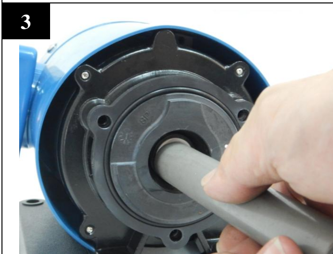
3 Press in the stationary part.
